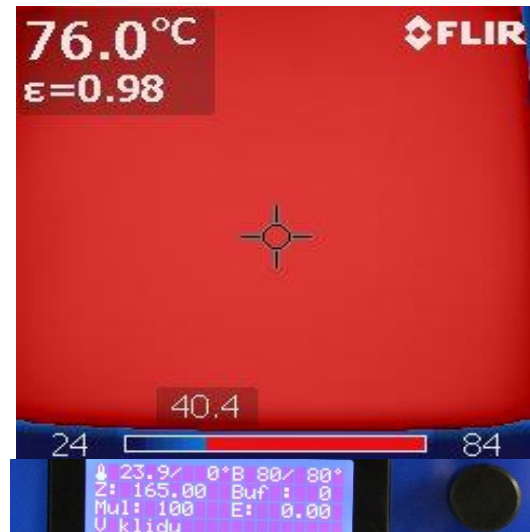
Figure 1 – Heated bed temperature – comparison between temperatures set to 80°C and the real state of temperature on the heated bed
